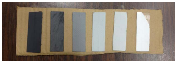
Figure 11. PVdF/PVP electrospun nanofibers with 0, 0.25, 0.5, 1, 2, and 4 wt % of carbon black (right to left). [Color figure can be viewed in the online issue, which is available at wileyonlinelibrary.com .]
